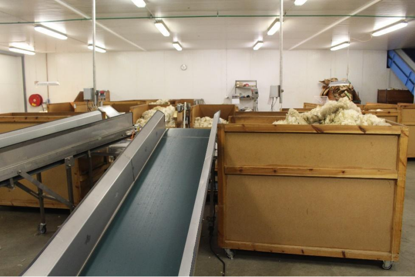
Figure 30: Wool sorting room at a slaughterhouse in Southern Norway: sheep ear tags are scanned and labels are printed giving the flock number and wool quality code, before being weighed and further sorted
