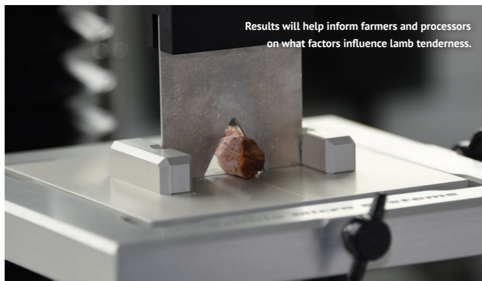
Cooked samples of Welsh Lamb are prepared at the laboratory for tenderness analysis.
